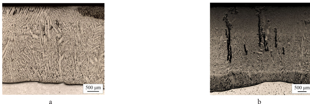
Fig. 3. (Color online) Structure of surfaced coatings based on Colmonoy-227F nickel alloy, formed using multi-layer cladding: double-layer surfacing (a), triple-layer surfacing (b).
