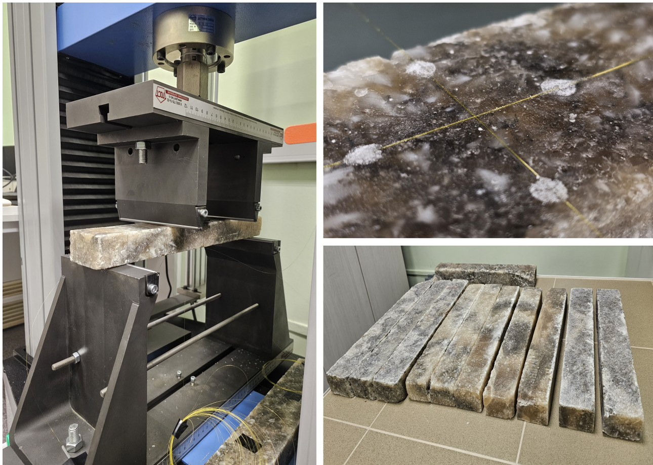
Fig. 2. (Color online) Universal four-point bending testing facility, fiber-optic sensors fixed on the sample surface, rock salt samples.
