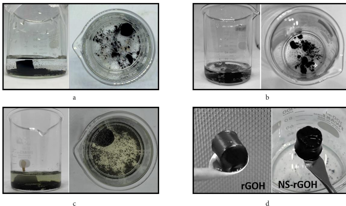
**Fig. S1.** (Color online) Photograph of rGOH (a), rGO (b), NS-rGOH (c) and the image of hydrogel structure (d).
