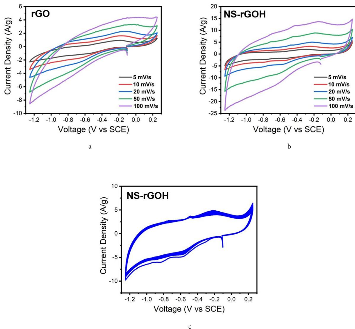
**Fig. S3.** (Color online) Cyclic Voltammetry curve of (a) rGO, (b) NS-rGOH in different scan rate, and (c) NS-rGOH for 10 cycles.
