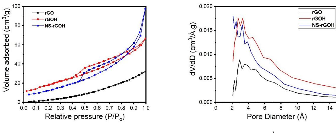
**Fig. S5.** (Color online) Nitrogen adsorption-desorption isotherms (a) and BJH pore size distribution of rGO, rGOH, and NS-rGOH.
