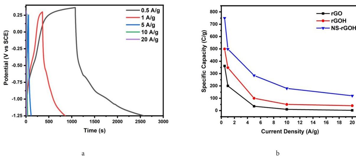
**Fig. S4.** (Color online) GCD Curves of NS-rGOH in various current density (a), specific capacity of rGO, rGOH and NS-rGOH in various current density (b).
