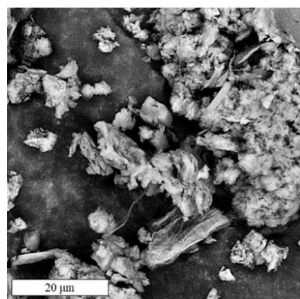
**Fig. S2.** SEM image of rGO sample.
