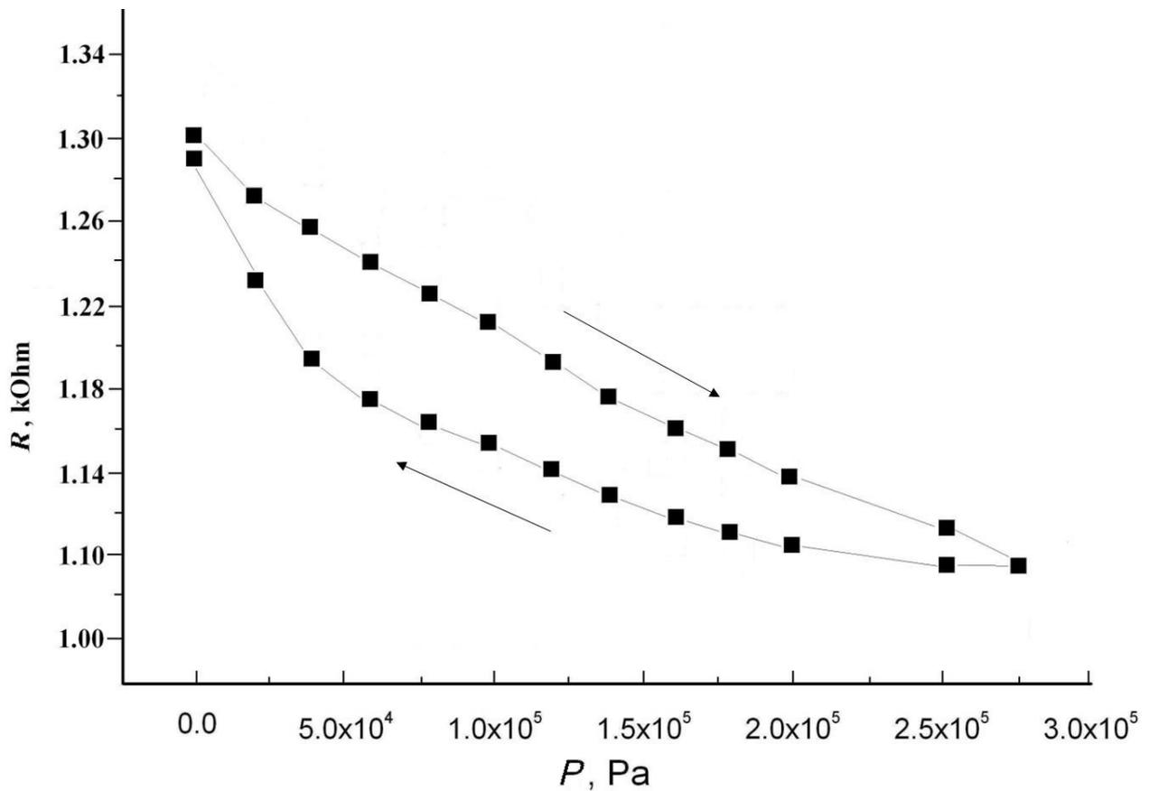
Fig. 55. Pressure dependence of the electrical resistance of the 15% LDPE/15% C/70% LSMO sample, PR=15.3%.
