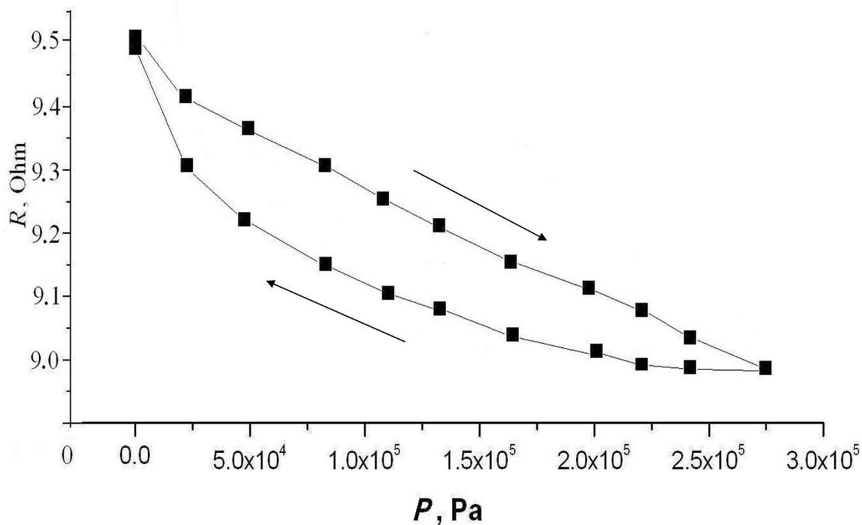
Fig. S3. Pressure dependence of the electrical resistance of the 15% LDPE/60% C/25% LSMO sample, PR = 6.1%.
