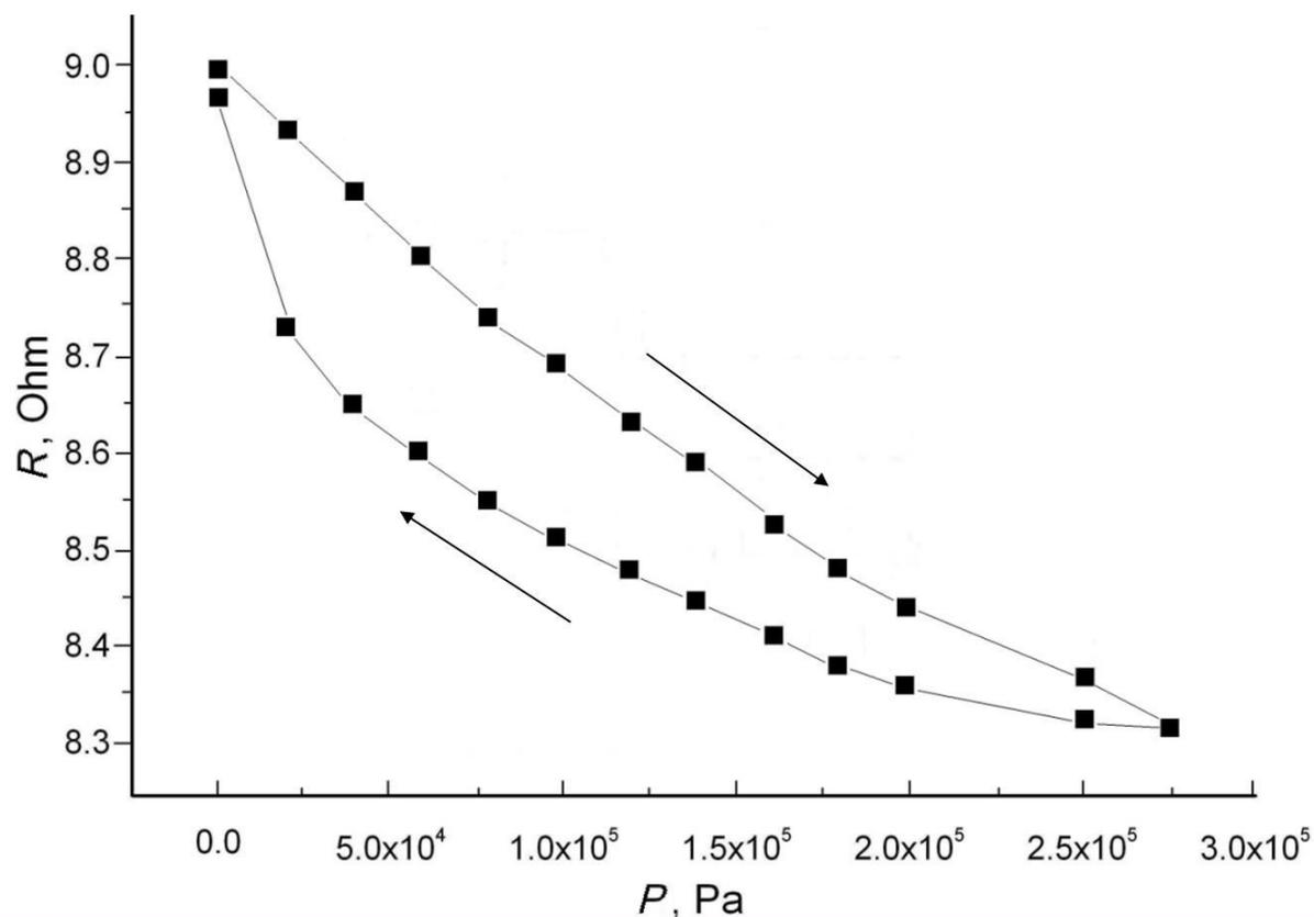
Fig. S2. Pressure dependence of the electrical resistance of the 15% LDPE/65% C/20% LSMO sample, PR = 7.5%.
