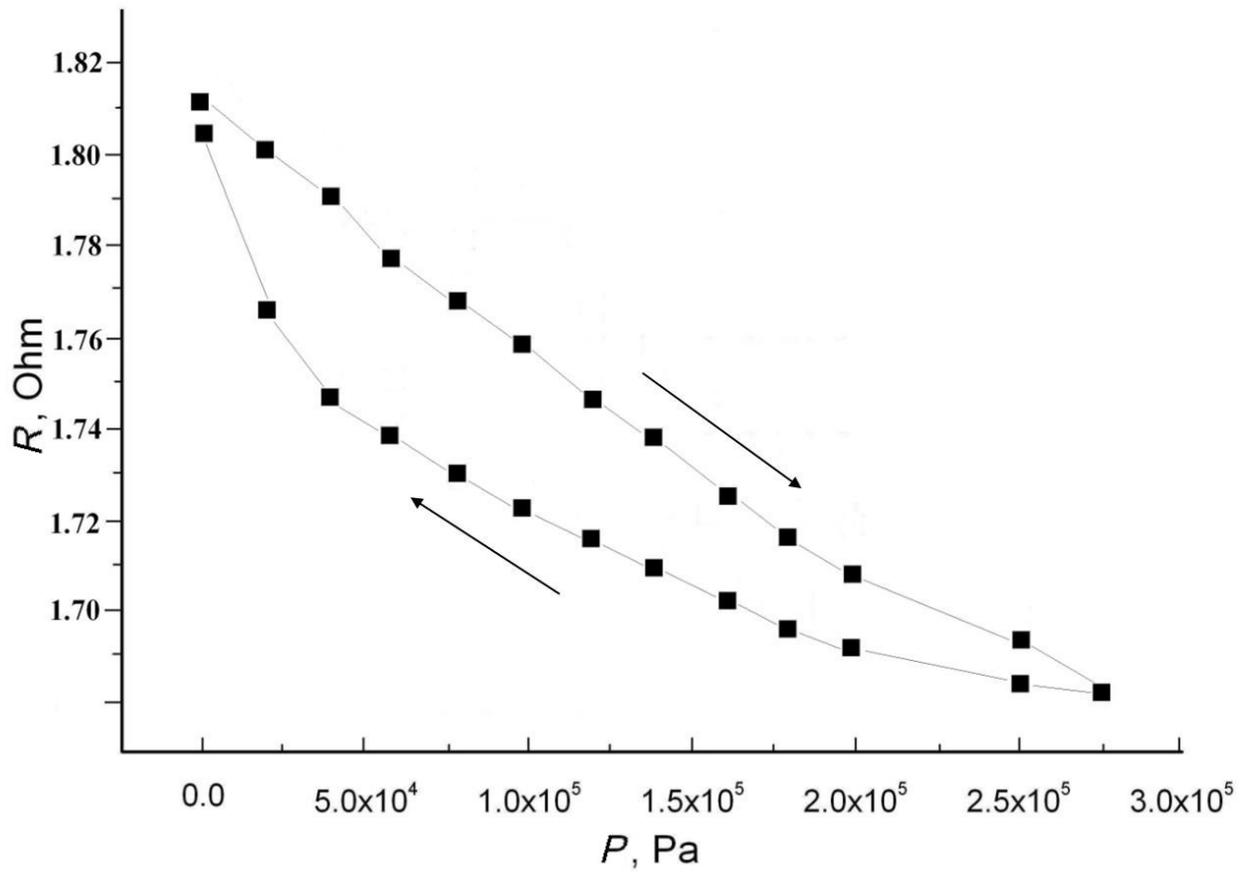
Fig. 54. Pressure dependence of the electrical resistance of the 15% LDPE/55% C/30% LSMO sample, PR=7.0%.
