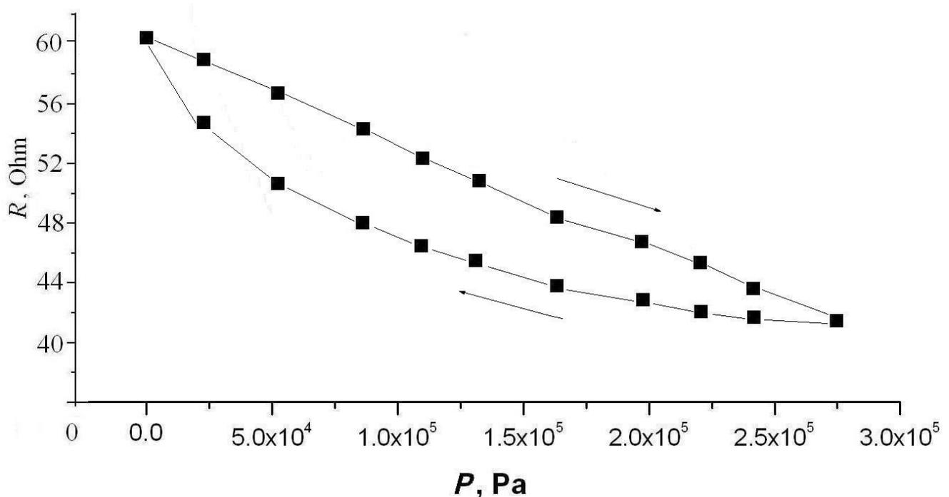
**Fig. S1.** Pressure dependence of the electrical resistance of the 15% LDPE/80% C/5% LSMO sample, PR = 30%.
