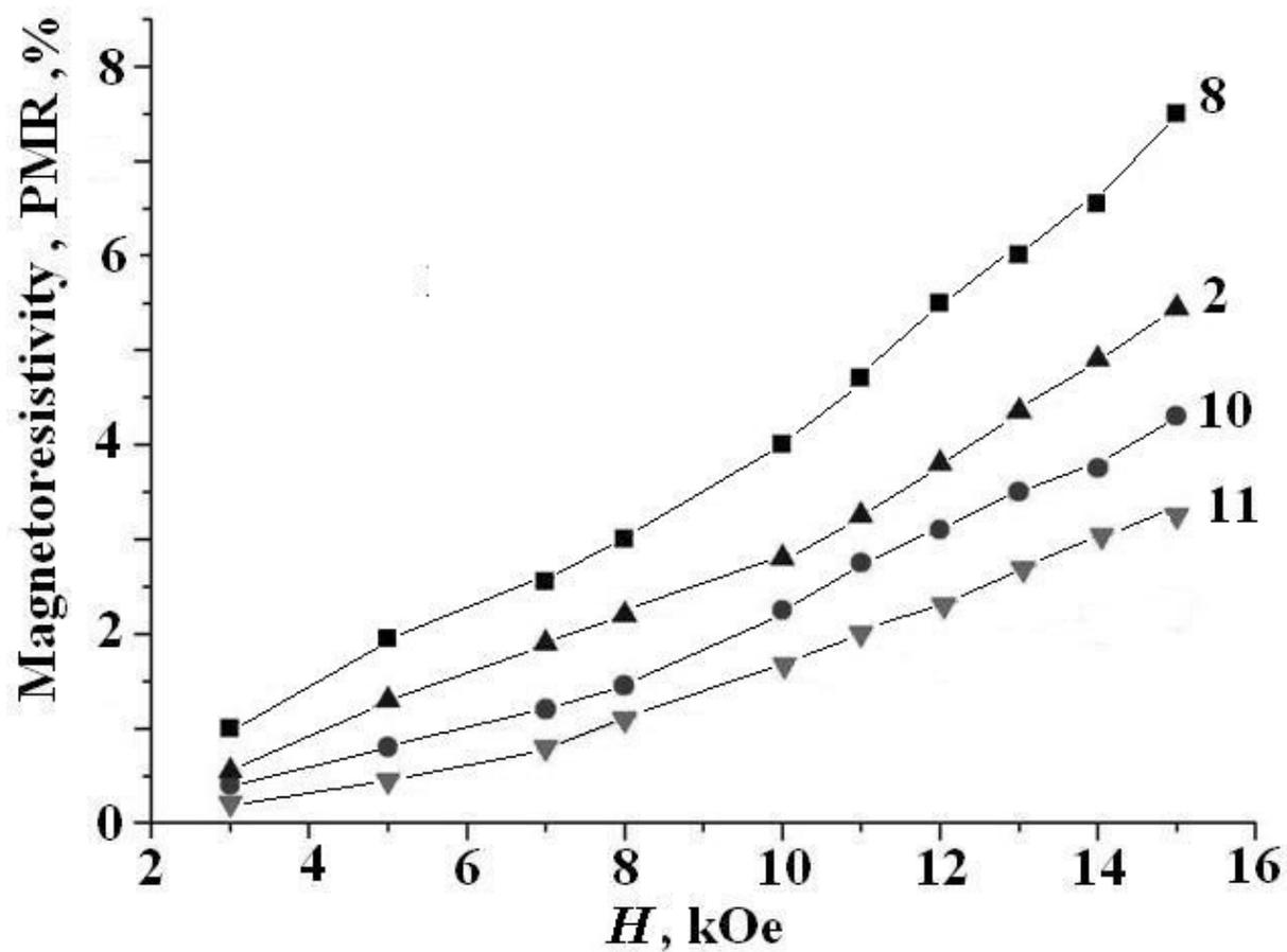
**Fig. 56.** Magnetoresistivity for a number of samples in constant magnetic field of different strength. Sample numbers correspond to the table in the article text.
