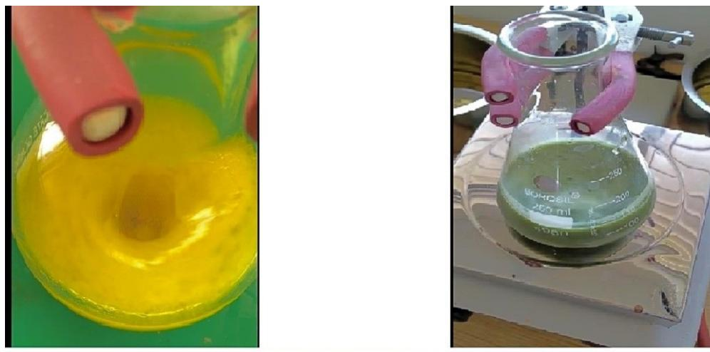
**Fig. 1S.** (Color online) Reaction illustrating synthesis of Cr nanoparticles in co-precipitation method (a) and precipitation of the Cr-WO<sub>3</sub> (15 wt.%) NPs (b).
