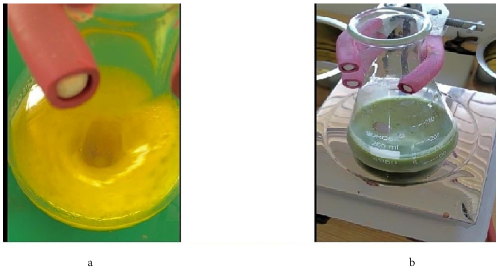
Fig. 15. (Color online) Reaction illustrating synthesis of Cr nanoparticles in co-precipitation method (a) and precipitation of the Cr-WO 3 (15 wt.%) NPs (b).
