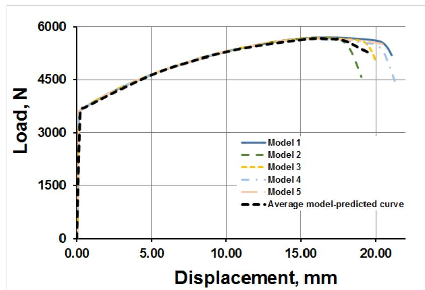
**Fig. S4.** The average model-predicted curve for nonhomogeneous specimens A.
