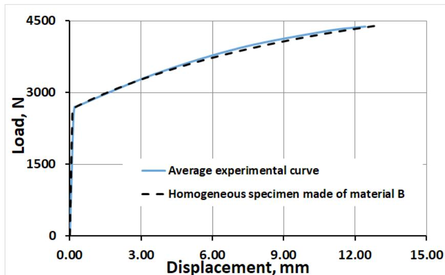
**Fig. S2.** Comparison of modeling results of a homogeneous specimen from material B with the average experimental curve.
