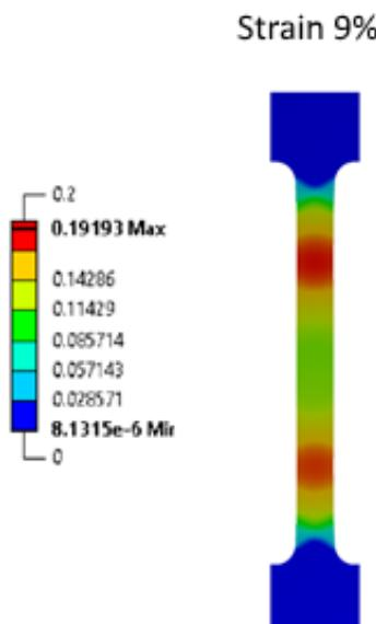
**Fig. S6.** Equivalent total strain at specimen elongation by 9%.
